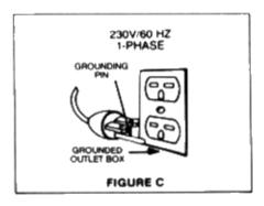
Always use a property grounded 3-wire extension cord which has male and female plugs. Use only 16-3 ST or SO type extension cords for a total cord length up to 75 feet.
