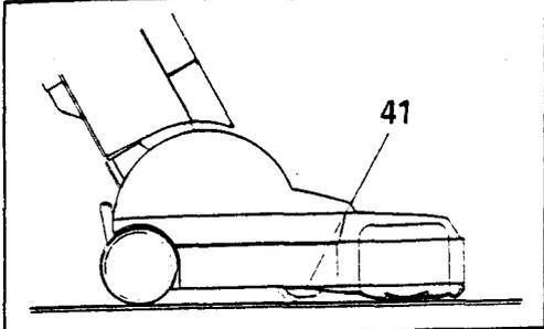
On hard floors the adjustment wheel (41), moves upwards into the machine so that the brush becomes flush with the floor. Therefore, the WINDSOR "SENSOR" can also be used to vacuum hard floors.
